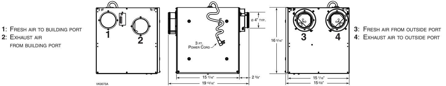
NOTE: ALL UNITS PORTS WERE CREATED TO BE CONNECTED TO DUCTS HAVING A MINIMUM OF 4" DIAMETER, BUT IF NEED BE, THEY CAN BE CONNECTED TO BIGGER SIZED DUCTS BY USING AN APPROPRIATE TRANSITION (E.G.: 4" DIAMETER TO 5" DIAMETER TRANSITION).
